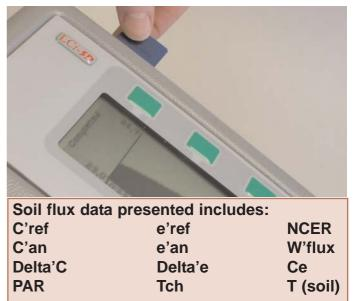
The SRS-*SD* series feature enhanced data capture and output capabilities. Experimental protocols, soil flux data and calculations are stored on easily exchangeable SD cards. This popular feature, already incorporated in other ADC gas exchange instrumentation, allows separate cards to be used by individual users or for specific experimental applications.
