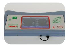
The LCi **7** provides unlimited data storage. All experimental protocols, data and calculations are stored on Secure Digital (SD) cards. SD cards can be interchanged for individual users or for specific experimental applications.
